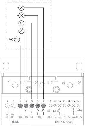
Figure 5.17: Terminals for status output signals
