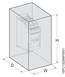
Figure 4.3: Dimensions minimum enclosure size
