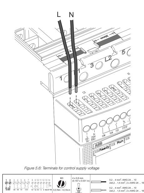
Figure 5.7: Tightening torques and wire area
