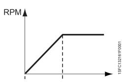
Figure 7.15: The function of Torque Control during start
