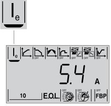
Figure 7.3: Rated Current parameter displayed
