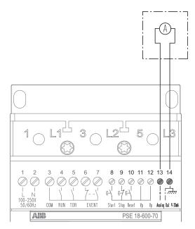
Figure 5.15: Terminals for analog output
