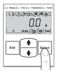
Figure 6.4: Reset of tripping events
