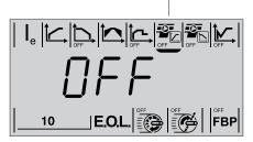
Figure 7.14: Torque Control during start ramp parameter displayed
