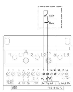
Figure 5.10: Terminals for start and stop, conventional circuit with push button
