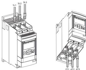
Figure 5.3: PSE18...PSE105 connection of the connection module line side and motor side terminals
