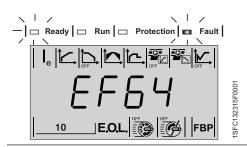
SF = Softstarter fault EF = External fault P = Protection
