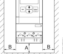
Figure 4.5: Minimum distances to wall and front
