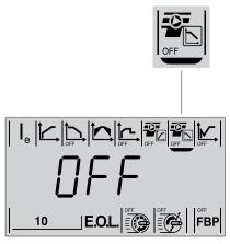
Figure 7.16: Torque Control during stop ramp parameter displayed
