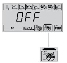
Figure 7.25: Locked Rotor Protection parameter displayed
