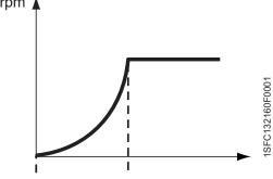
Figure 7.5: The function of Start Ramp Time
