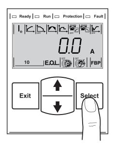
Figure 7.32: Reset of tripping events
