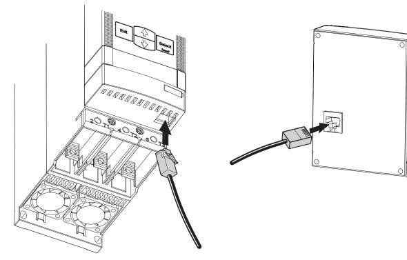
Figure 5.20: Connection of external keypad
