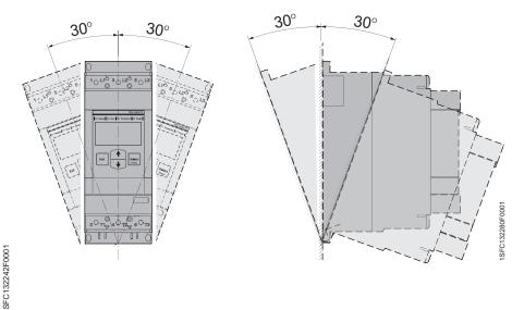
Figure 4.6: Maximum mounting angle
