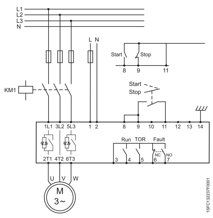
Circuit diagram PSE18...PSE370 (Fuse and contactor version)
