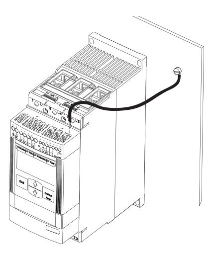
Figure 5.8: Terminal for functional earth
