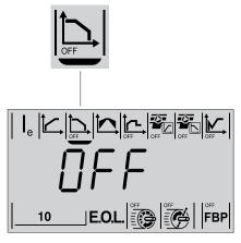
Figure 7.6: Stop Ramp Time parameter displayed
