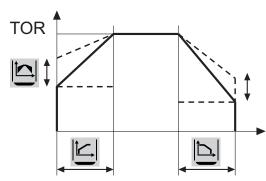
Figure 7.9: The function of Initial/End Voltage
