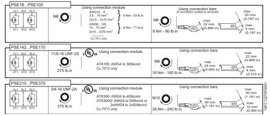
Figure 5.5: Tightening torques and dimensions for terminal bars and lugs
