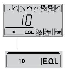
Figure 7.20: Electronic Motor Overload Protection EOL parameter displayed
