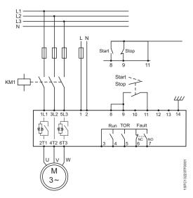
Figure 2.2: Example connection of PSE Softstarter
