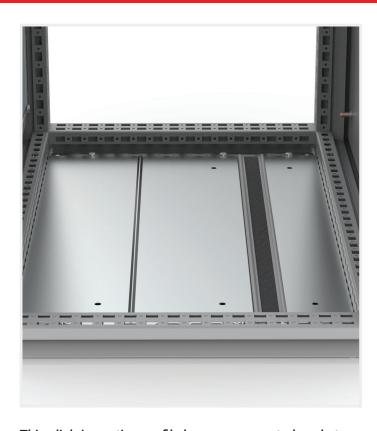
This click-in section profile has a pre-mounted gasket to seal the empty space around cables routed between bottom plates, which maintains the enclosure's protection degree.
